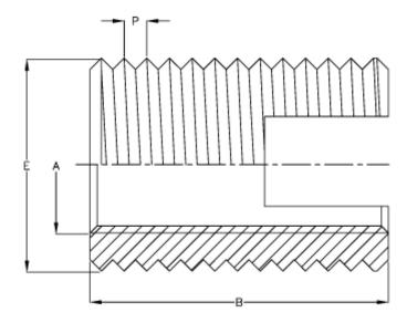
Female thread A = M12 Length B = 22 Male thread E = 16.0 Min hole depth blind hole = 26
